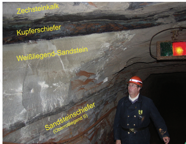
Figure 3. The upper Permian-lower Triassic sequence is from upper (Sandsteinschiefer) Rotliegend sandstone in the footwall, the mineralized Weissliegend white sandstone and Kupferschiefer metallized black shale, and the hanging wall of Zechstein dolostone. Location: Roerigschacht, Wettelrode/Sangerhausen mine, Mansfeld district, Germany. The Permo-Triassic boundary is placed at the Kupferschiefer-Zechstein contact. (Photo by Juergen Kopp showing the mine manager Dipl.-Ing. Erich Hartung).
